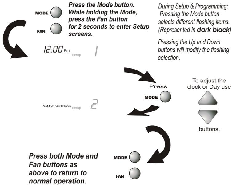
The thermostat is preprogrammed from the factory to operate 1 or 2 Stage equipment\* without the need for further programming. To optimize the installation of this thermostat follow the instructions in the Advanced Setup section.
