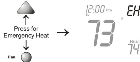
During Emergency Heat the thermostat will turn on the fan and the 2nd stage of heat, when there is a demand for heat, locking out the 1st stage compressor. Exiting Emergency Heat is the same as entering. During Emergency Heat only OFF and HEAT are available.
