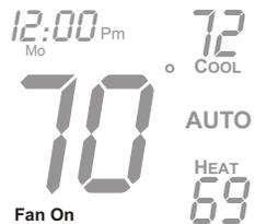
**Fan On** indicates constant fan operation. This feature is active even if the thermostat is set to **Off**.
