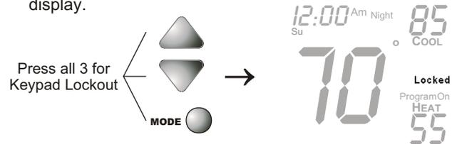
To **unlock** the buttons, again press and hold the Mode button. While holding the Mode button in, press the Up and Down buttons in together. The **Locked** icon will disappear from the display.
