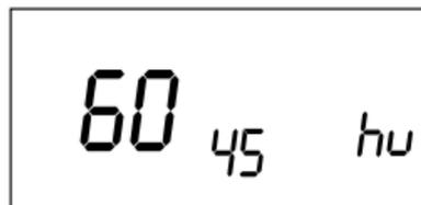
The current indoor humidity (large number) and humidify set point (small number) are displayed along with the humidify indicator (hu).
