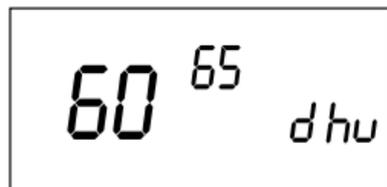
The current indoor humidity (large number) and dehumidify set point (small number) are displayed along with the dehumidify indicator (dhu).
