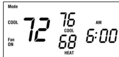
When the ON mode is selected, the fan runs continuously for improved air circulation.
